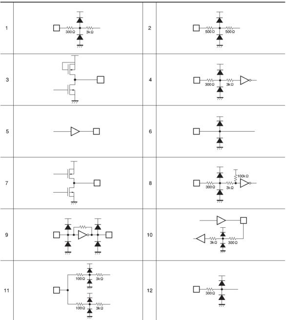
\*1 MIRROR, SCRATCH, FOK, SUBCK, MCK, DIN, RW, RESET, EXPLCK, EYE, DECTR, DFLRCK, DFDIN, DFDCK \*2 FON, RFCK, WFCK, SUBSYQ, SUBDATA, DOUT, BUSY, XOUT, SENS, GFS, ASY, C1F1, C1F2, C2F1, C2F2, C2CLK, C2F, DE, LRCK, DOCK, CLK \*3 RESET \*4 PLLSW, TCAPA2, FSW \*5 FEIN, TEIN
