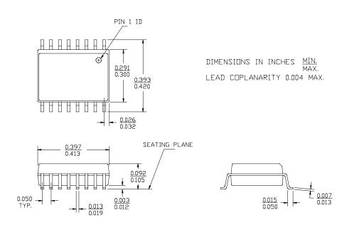
16-Lead Molded SOIC S1
