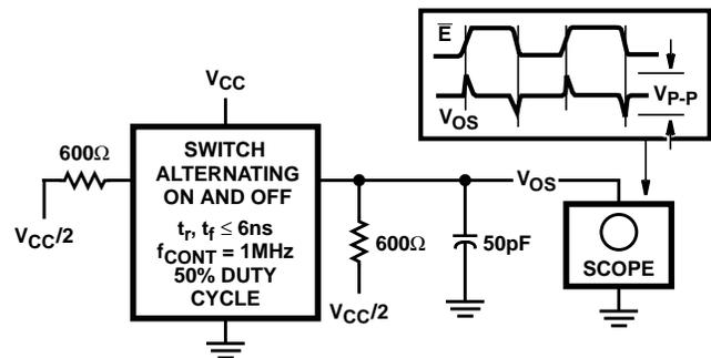
FIGURE 6. CONTROL TO SWITCH FEEDTHROUGH NOISE TEST CIRCUIT
