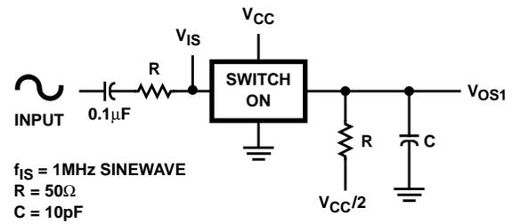
FIGURE 4. CROSSTALK BETWEEN TWO SWITCHES TEST CIRCUIT
