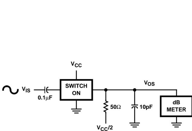
FIGURE 3. FREQUENCY RESPONSE TEST CIRCUIT
