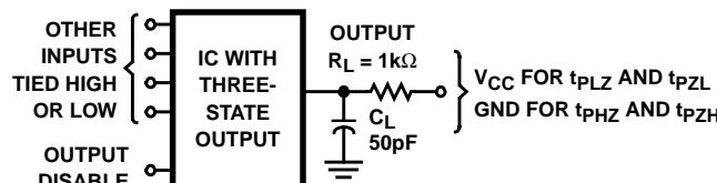
NOTE: Open drain waveforms  $t_{PLZ}$  and  $t_{PZL}$  are the same as those for three-state shown on the left. The test circuit is Output  $R_L = 1\text{k}\Omega$  to  $V_{CC}$ ,  $C_L = 50\text{pF}$ .
