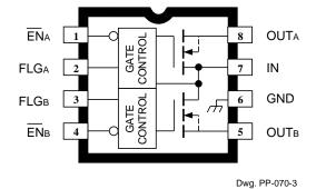
Note that the A2536EM (DIP) and the A2536EL (SOIC) are electrically identical and share a common terminal number assignment.
