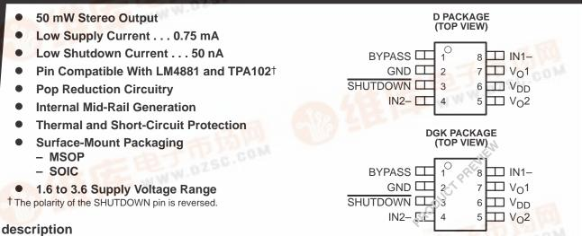
The TPA6100A2 is a stereo audio power amplifier packaged in either an 8-pin SOIC package or an 8-pin MSOP package capable of delivering 50 mW of continuous RMS power per channel into 16- $\Omega$  loads. Amplifier gain is externally configured by a means of three resistors per input channel and does not require external compensation for settings of 1 to 10.
