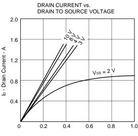
V<sub>DS</sub> - Drain to Source Voltage - V
