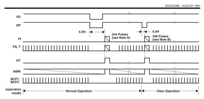
NOTES: A. When VD is low and GP goes low, 244 pulses are generated on PI, PS, and T.
