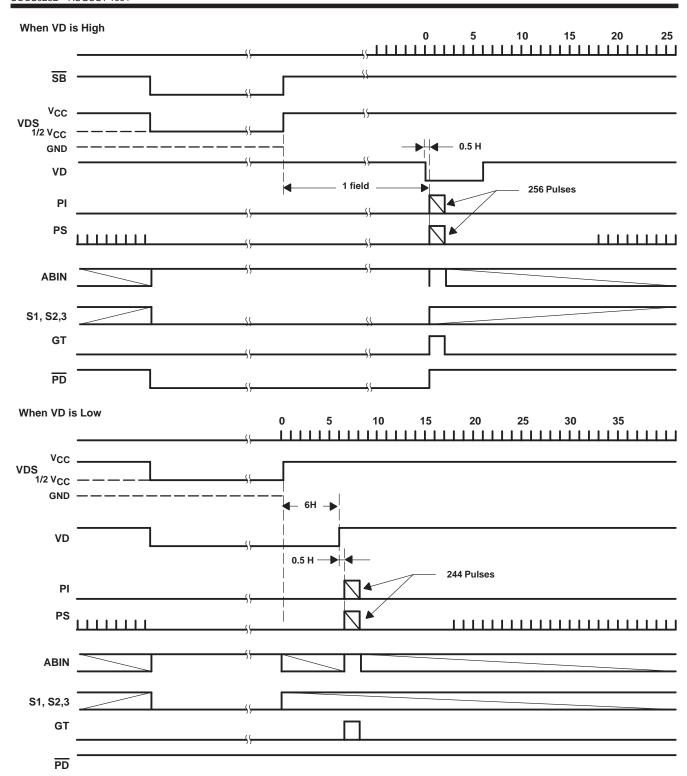
Figure 8. Timing for VDS in the Reset Mode
