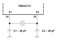
NOTE: The TMS3471C is designed for use with a crystal oscillator. The X1 and X2 terminals should not connect directly to external driver outputs.
