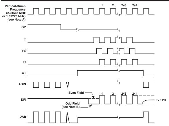
NOTES: A. When the vertical-dump frequency is 1.02273 MHz, PI, PS, and T have a 50% duty cycle.
