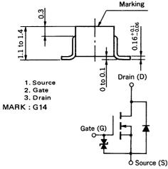
(Diode in the figure is the parasitic diode.)
