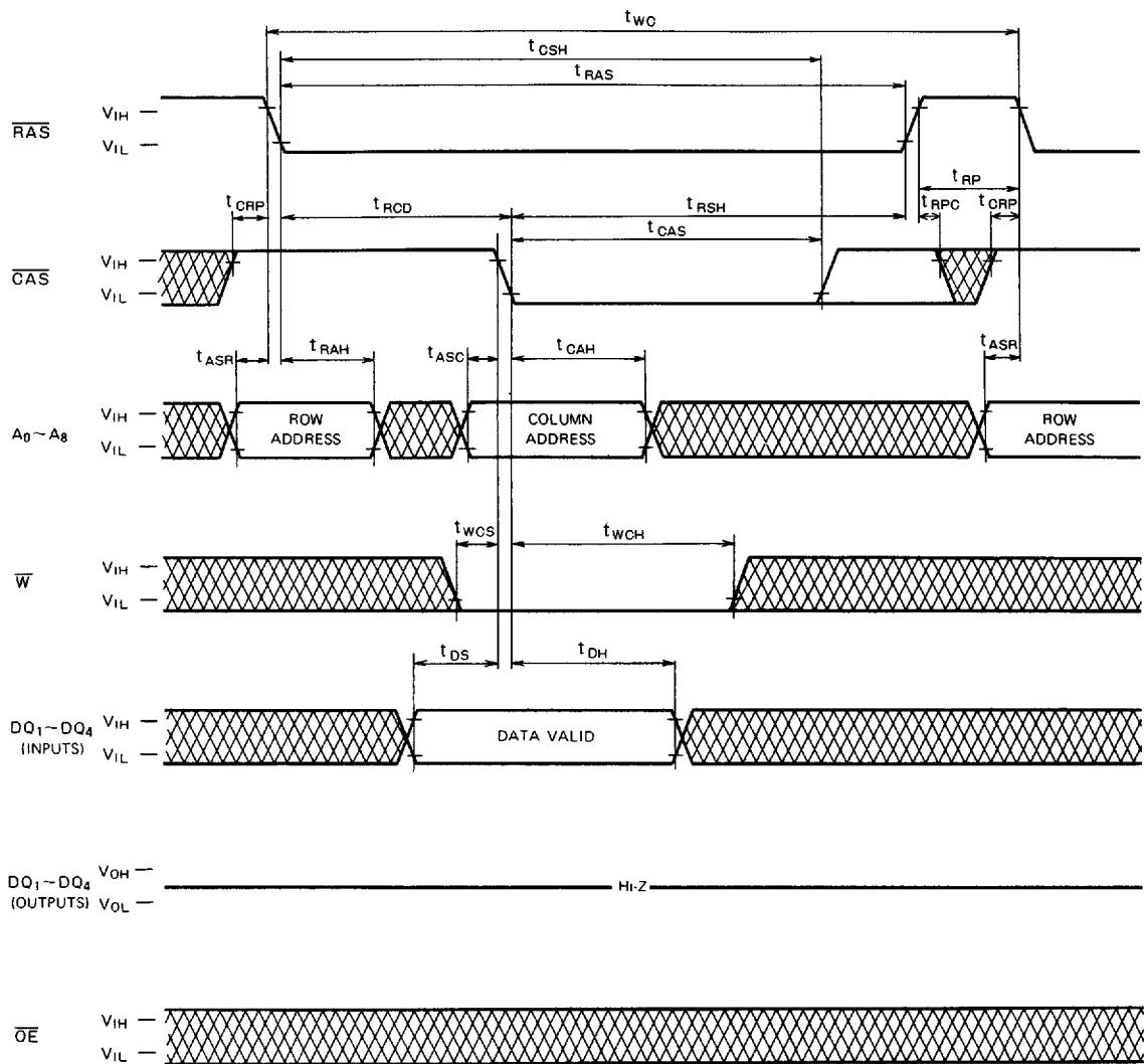
**M5M44256BP,J,L,VP,RV-7,-8,-10****FAST PAGE MODE 1048576-BIT(262144-WORD BY 4-BIT)DYNAMIC RAM****Write Cycle (Delayed Write)**
