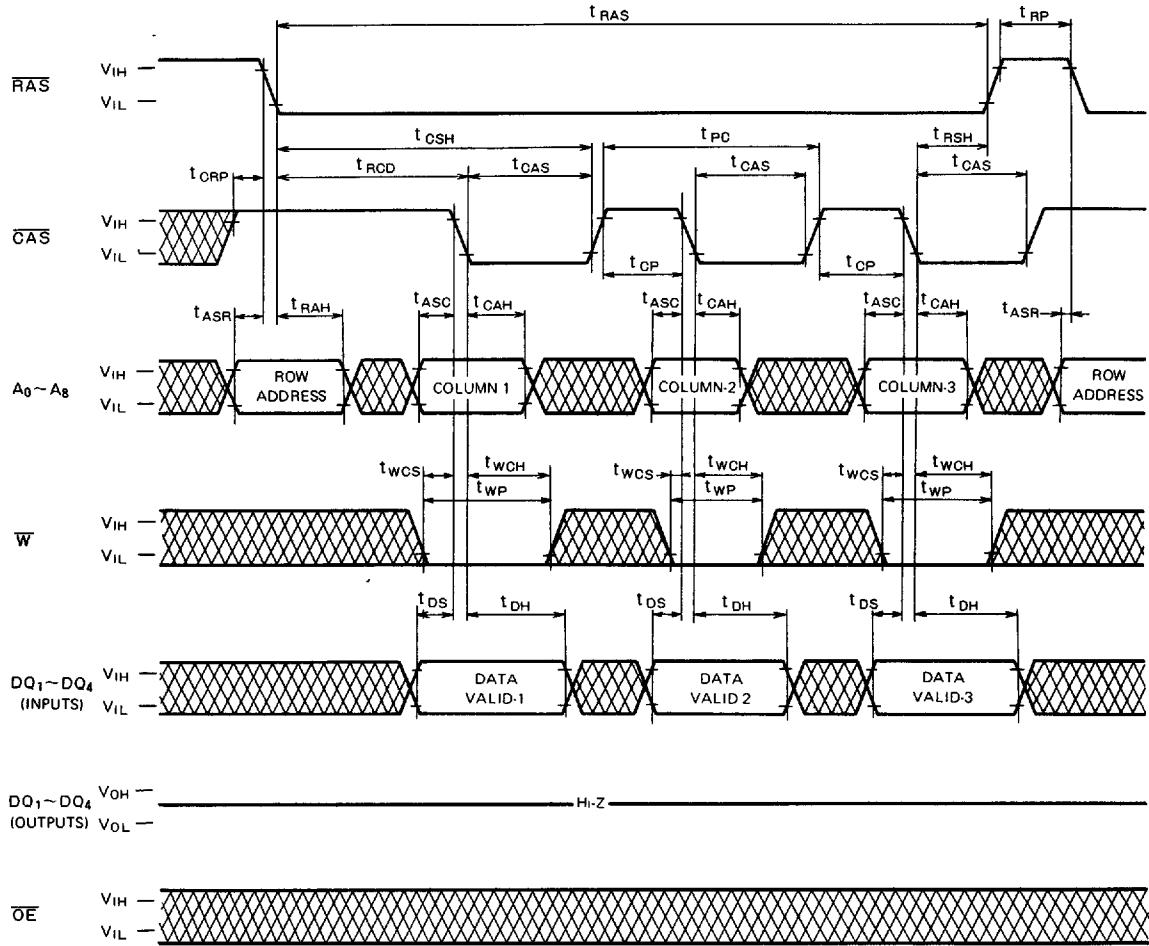
**FAST PAGE MODE 1048576-BIT(262144-WORD BY 4-BIT)DYNAMIC RAM****Fast Page Mode Write Cycle (Delayed Write)**
