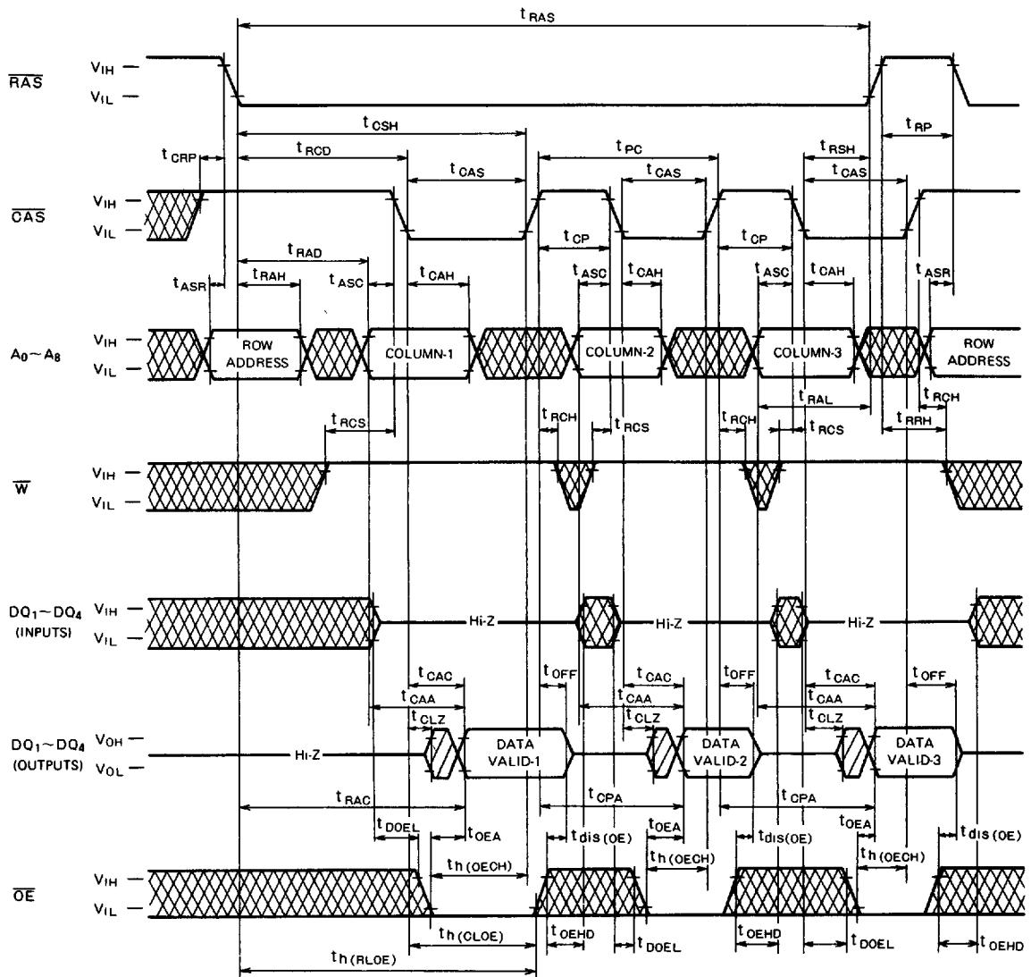
**FAST PAGE MODE 1048576-BIT(262144-WORD BY 4-BIT)DYNAMIC RAM****Fast Page Mode Write Cycle (Early Write)**
