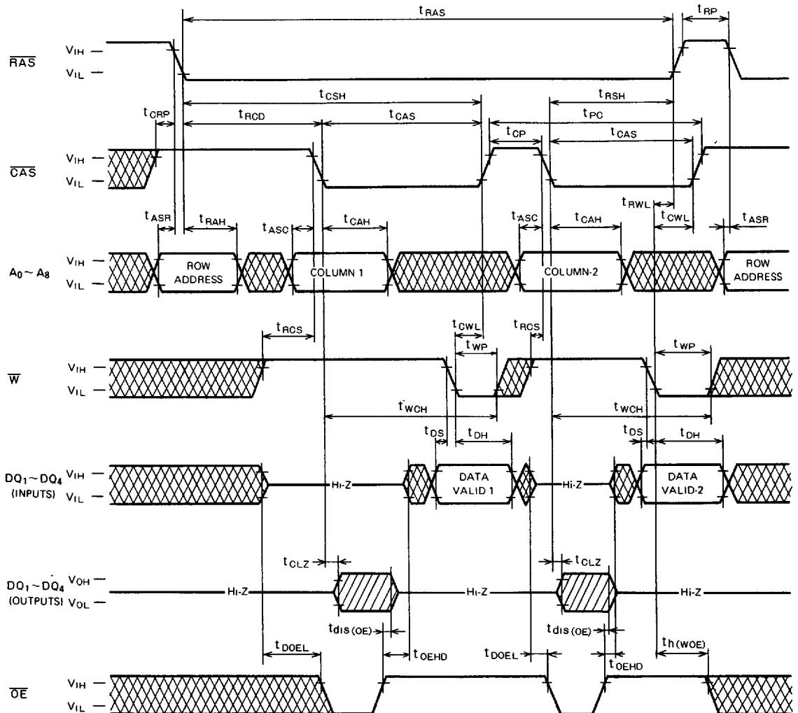
**FAST PAGE MODE 1048576-BIT(262144-WORD BY 4-BIT)DYNAMIC RAM****Fast Page Mode Read-Write, Read-Modify-Write Cycle**
