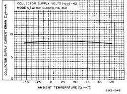
Fig.11 - Collector Supply Current Drain (12) vs Ambient Temperature
