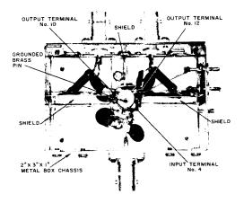
Fig.6 - Test Circuit Layout
