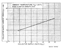
Fig.10 - Collector Supply Current Drain (12) vs Collector Supply Voltage (VCC)
