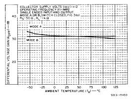
Fig.12 - Single-Ended Differential Voltage Gain vs Ambient Temperature
