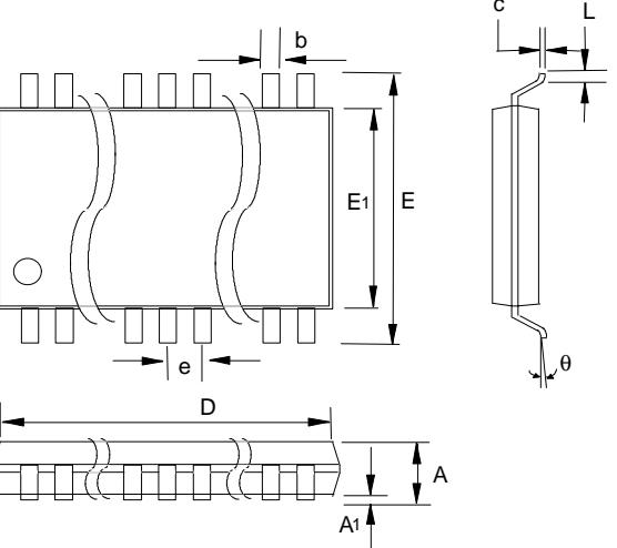
The diagram shows a top-down view of a 20-pin TSSOP package. It features a rectangular body with a row of 20 pins on one side. Key dimensions are labeled: D (total width), E (total height), E1 (height of the body), b (width of the pins), c (width of the lead), L (lead length), and θ (lead pitch). A1 is the height of the lead above the body. The package is shown in two orientations: one with pins facing right and one with pins facing left.
