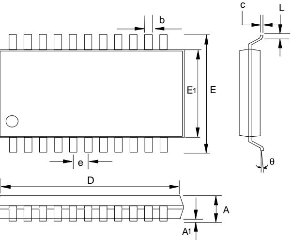
The diagram shows a top-down view of a 20-pin SOP package. It features a rectangular body with a row of 20 pins on one side. Key dimensions are labeled: D (total width), E (total height), E1 (height of the body), b (width of the pins), c (width of the lead), L (lead length), and θ (lead pitch). A1 is the height of the lead above the body. The package is shown in two orientations: one with pins facing right and one with pins facing left.
