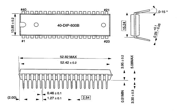
NOTE: Dimensions are in millimeters.
