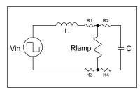
Figure 1, Dimming ballast output stage.
