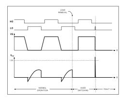
Figure 18, hard-switching with latch off
