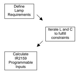
Figure 19, Simplified Ballast Design Procedure
