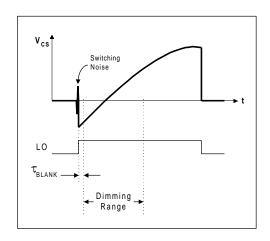
Figure 15, Current sense timing diagram.
