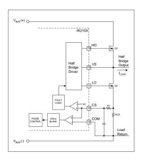
Figure 14, Current sensing circuitry.
