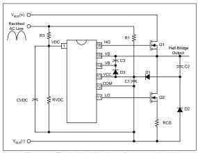
Figure 5, Typical application of start-up circuitry.
