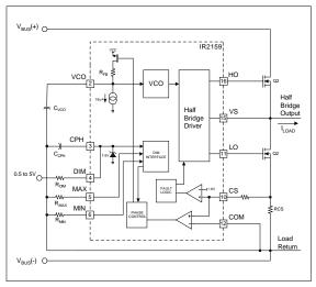
Figure 11, IR2159 dimming circuitry.
