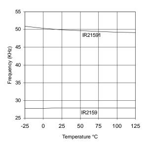
Graph 15. Frequency vs Temperature V<sub>VCO</sub>= 0V (IR2159/IR21591)
