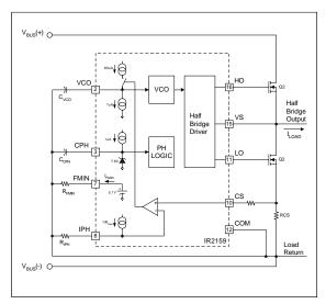
Figure 7, IR2159 preheat circuitry.
