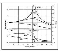
Figure 2, Typical output stage transfer function for different lamp power levels.
