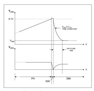
Figure 10, IR2159 ignition timing diagram.
