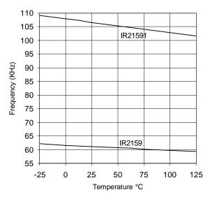
Graph 16. Frequency vs Temperature V<sub>VCO</sub>= 2V (IR2159/IR21591)
