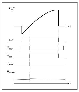
Figure 12, Phase control timing diagram.
