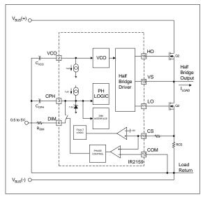
Figure 9, IR2159 ignition circuitry.
