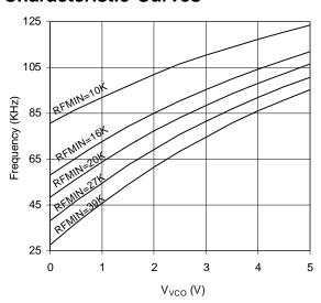
Graph 1. Frequency vs  $V_{VCO}$  (IR2159)
