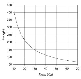
Graph 7. I<sub>MIN</sub> vs R<sub>FMIN</sub> (IR2159/IR21591)
