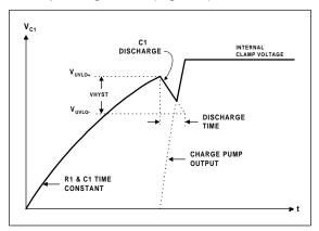
Figure 6, Start-up capacitor (C1) voltage.
