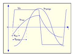
Figure 3, Typical ballast output stage waveforms.
