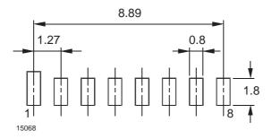
Figure 10. TFDT4500 Top View Package Note: Leads of the device should be at least 0.3 mm within the ends of the pads. Pad 1 is longer to designate Pin 1 connection to transceiver.
