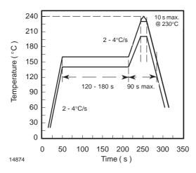
Figure 11. Recommended Solder Profile
