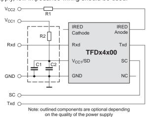
Figure 3. Recommended Application Circuit
