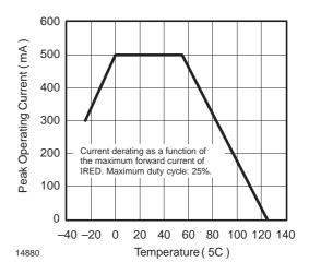
Figure 12. Current Derating Diagram
