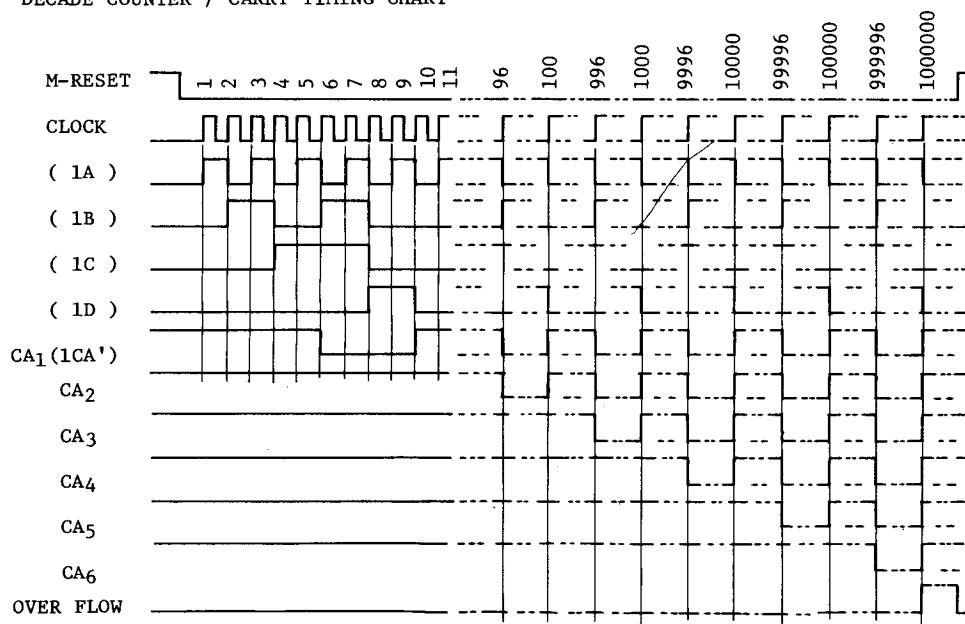
\* Waveform marked with ( ) are timings of LSI's internals.(Refer to LOGIC DIAGRAM)
