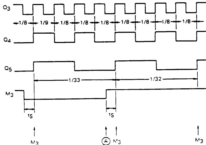
When both  $Q_4$  and  $Q_5$  are low level, the  $M_3$  pin is active. If the  $M_3$  pin is low at (A) point, the division ratio is  $1/9$ , otherwise the division ratio is  $1/8$ . So  $1/33$  division ratio means  $N = 9 \times 1 + 8 \times 3$ .
