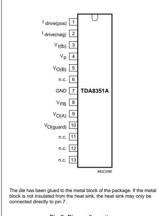
Fig.2 Pin configuration.
