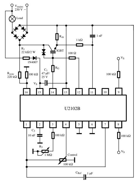
Figure 12. Reverse phase control for ac loads
