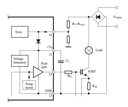
Figure 4. Power supply for dc loads (R<sub>1</sub> is identical with R<sub>sync</sub>)
