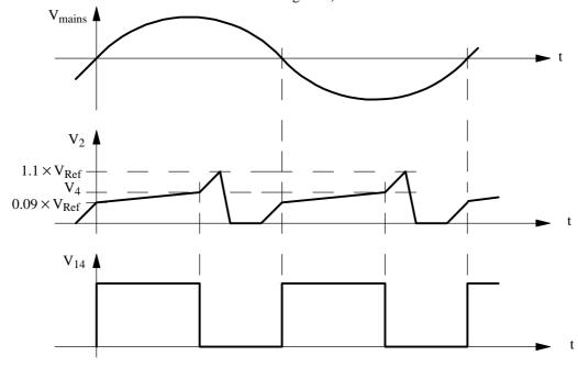
Figure 7. Signal characteristics of reverse phase control
