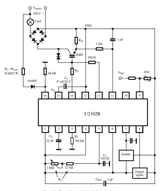
Figure 11. Zero voltage switch mode for ac loads
