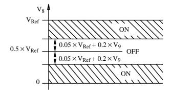
Figure 9. Trigger condition Pin 8
