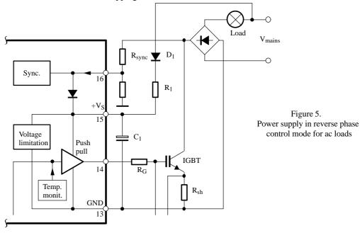
In two-wire systems, the additional power supply at Pin 15 is not possible (see figure 4, by omitting  $R_1$  and Diode  $D_1$ ). In this case, the resistor  $R_{sync}$  is identical with  $R_1$  and should be as low as the power dissipation allows it. A sufficiently large residual phase angle must remain in this case in order to guarantee the device supply.
