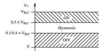
Figure 8. Trigger condition Pin 7
