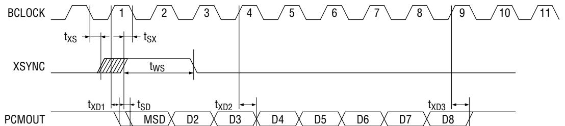
When  $t_{XS} \leq 1/2 \cdot F_c$ , the Delay of the MSD bit is defined as  $t_{WD1}$ .
