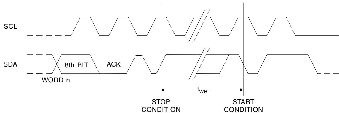
Note: Note: The write cycle Time  $t_{WR}$  is the time from valid stop condition of a write sequence to the end of the internal clear/write cycle.
