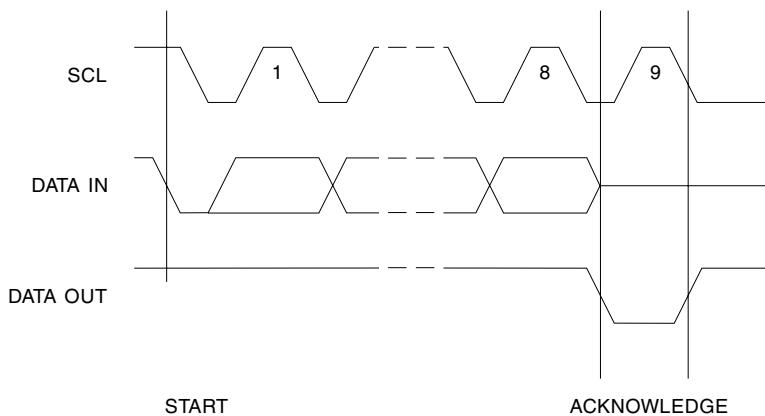
Note: To transmit a NACK (no acknowledge), hold data (SDA) high during the entire 9<sup>th</sup> clock cycle.
