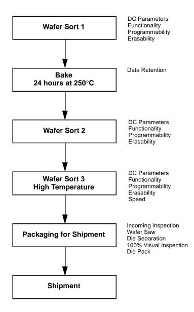
Figure 1. AMD KGD Product Test Flow
