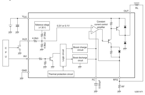
[Boost charge and discharge circuits]
