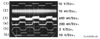
FIGURE 24. Oscillogram revealing signals at several important nodes under weak signal (0.5 mV<sub>RMS</sub>) conditions with SCR spikes on an otherwise quiet 115 V, 60 Hz power line. The signals are: 1) transmitted data, 2) RX carrier on the tuned transformer, 3) demodulated signal from the PLL after passing thru circuit of *Figure 22*, 4) signal after RC lowpass, 5) data at impulse noise filter integrator, and 6) received data. Horizontal scale is 10 ms per div.
