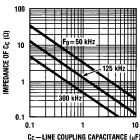
FIGURE 9. C<sub>C</sub>'s impedance should be, as a rule-of-thumb, smaller than the lowest expected line impedance
