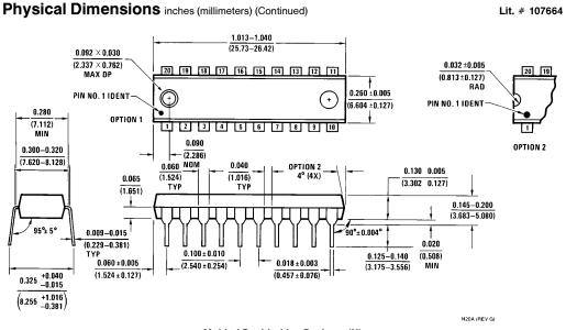
Molded Dual-In-Line Package (N) Order Part LM2893N NS Package Number N20A
