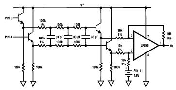
FIGURE 22. Circuit to view the differential demodulated data signal, minus the noise and 2F<sub>O</sub> components, conveniently with a single-ended gain-of-one output
