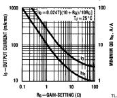
FIGURE 11. Output amplifier current and required min. Q<sub>B</sub> h<sub>fe</sub> versus gain-setting resistor R<sub>G</sub>
