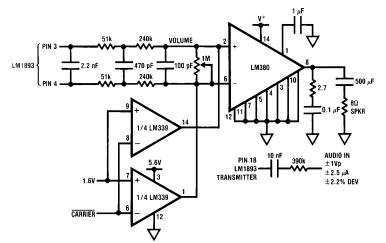
FIGURE 31. A simple linear analog audio transmitter and receiver are shown. The carrier and 1.6V inputs are derived from the carrier detector of *Figure 30*. The remaining 2 LM339 comparators may be used to build the carrier detector circuit.
