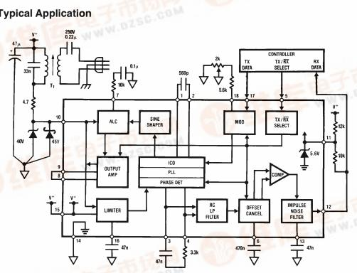
FIGURE 1. Block diagram of carrier—current chip with a complement of discrete components making a complete F<sub>O</sub> = 125 kHz, f<sub>DATA</sub> = 360 Baud transceiver. Use caution with this circuit—dangerous line voltage is present.
