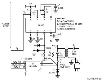
FIGURE 30. A simple carrier amplitude detector with output low when carrier is detected
