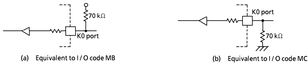
Figure 1-2. I/O code and external circuitry
