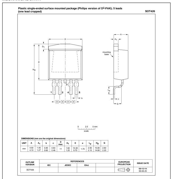
Fig.4. SOT426 surface mounting package<sup>1</sup>, centre pin connected to mounting base.
