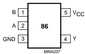
Fig.1 Pin configuration.
