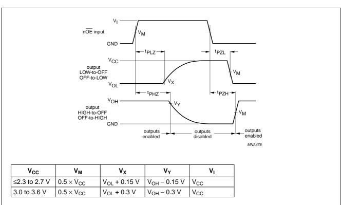
$V_{\mbox{\scriptsize OL}}$  and  $V_{\mbox{\scriptsize OH}}$  are typical output voltage drop that occur with the output load.
