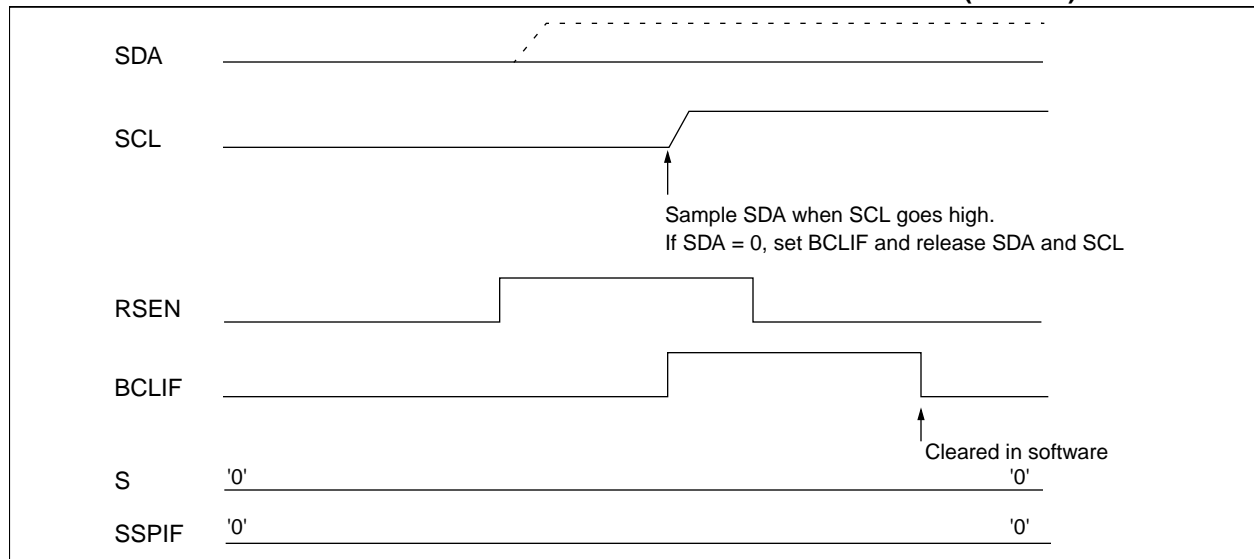
FIGURE 9-38: BUS COLLISION DURING A REPEATED START CONDITION (CASE 1)
