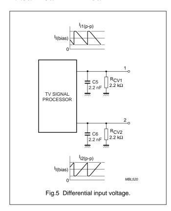
Values for these currents are, for instance:  $I_{i(bias)} = 400 \ \mu A; \ I_{i1(p-p)} = I_{i2(p-p)} = 475 \ \mu A.$
