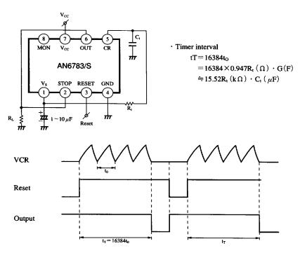
Note) The AN6784 can be also applied as the above, when the terminal functions are matched.
