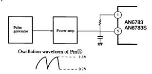
Frequency higher than that of oscillation at C, R is inputted to Pin 5 to shorten the timer interval. At this time, since capacitor of large capacitance is attached to the Pin 5, the power amp. with output of totem pole type should be used (not required if the output of pulse generator is large enough). However, arrangement should be made so that the input waveform could not exceed 1.8V.
