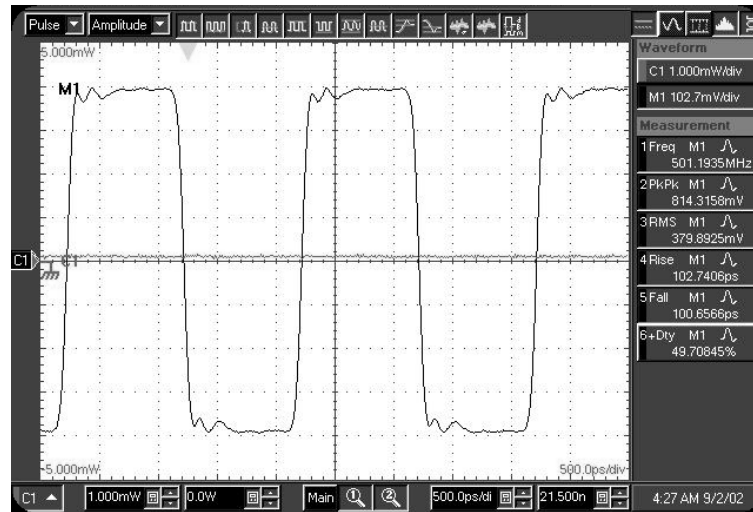
Figure 13 - Differential output with lower frequency input VCC = 4.75V, Vin = 10dBm, Fin = 2GHz
