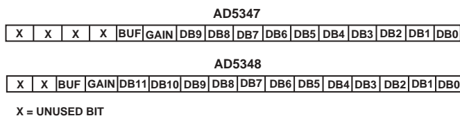
Figure 10. AD5347/AD5348 Data Format for Word Load with GAIN and BUF Data on 16-Bit Bus
