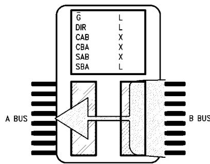
Note 2: The complement of A and B data are stored and transferred for DM74AS648
