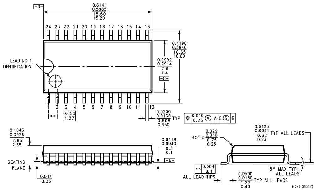
24-Lead Small Outline Integrated Circuit (SOIC), JEDEC MS-013, 0.300 Wide
