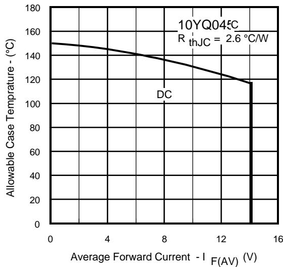
Fig. 5 - Max. Allowable Case Temperature Vs.
