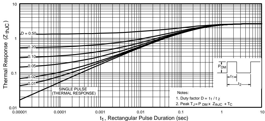
Fig. 4 - Max. Thermal Impedance  $Z_{thJC}$  Characteristics
