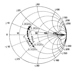
$\begin{array}{l} S21e: V_{CE}\,{=}\,10V \\ f\,{=}\,100MHz, 200 \text{ to } 1200MHz \,(200MHz \, step) \end{array}$
