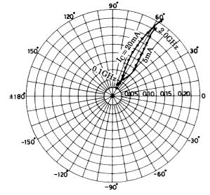
$\begin{array}{l} S22e: V_{CE}\!=\!5V \\ f\!=\!100MHz, 200 \text{ to } 2000MHz \text{ } (200MHz \text{ } step \text{ }) \end{array}$
