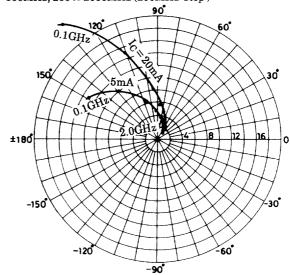
$\begin{array}{l} S12e:V_{CE}\!=\!5V\\ f\!=\!100MHz, 200\,\mathrm{to}\,2000MHz\,(200MHz\ step\,) \end{array}$
