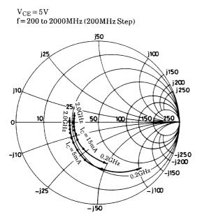
$V_{CE} = 5V$ f = 200 to 2000MHz (200MHz Step)
