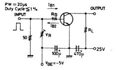
I C=10 I B1=-10 I B2=500mA, VCC=25V (For PNP, the polarity is reversed.) Unit (resistance : Ω, capacitance : F)
