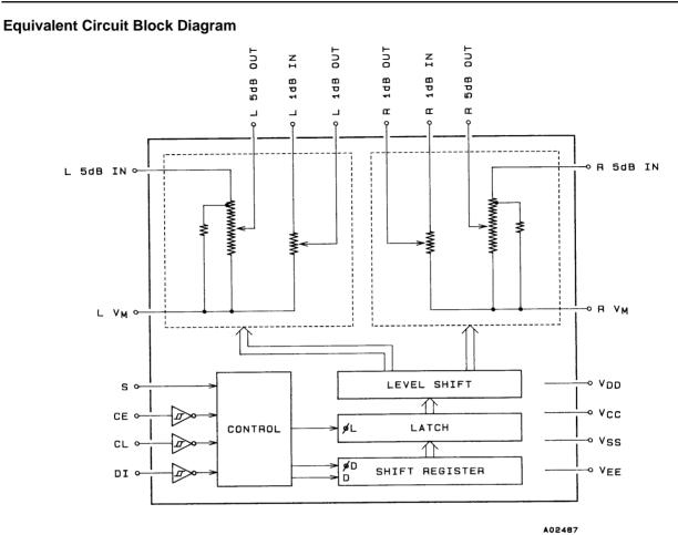
Internal Resistor Equivalent Circuit Diagram
