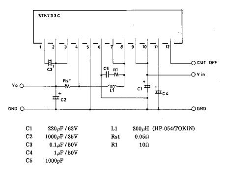
Note) Since the 5 pin is grounded to the substrate, these are influenced by noise when the radiator is connected to the circuit of the FG and GND lines. Under such conditions, the radiator should either be floated or an insulated seating used.
