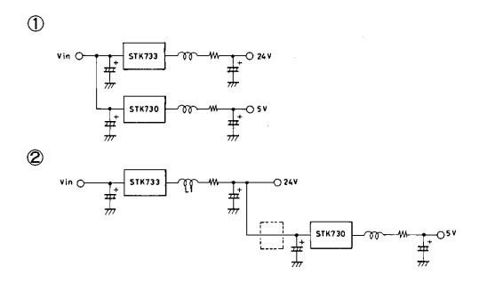
(Note) Due to the negative influences the 24 V system receives from the STK730 input ripple current and the assertion of L1, L should be installed in the [\_\_\_\_] section and the formation of a LC filter.
