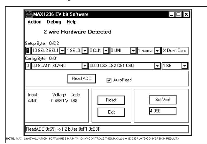
Figure 1. MAX1236 EV Kit Software Main Window
