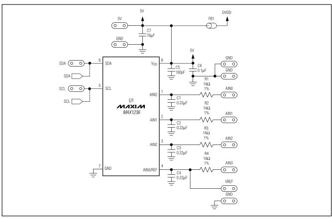
Figure 2. MAX1236 EV Kit Schematic (Sheet 1 of 2)
