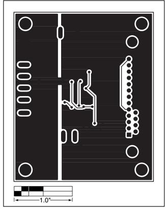
Figure 5. MAX1236 EV Kit PC Board Layout—Solder Side
