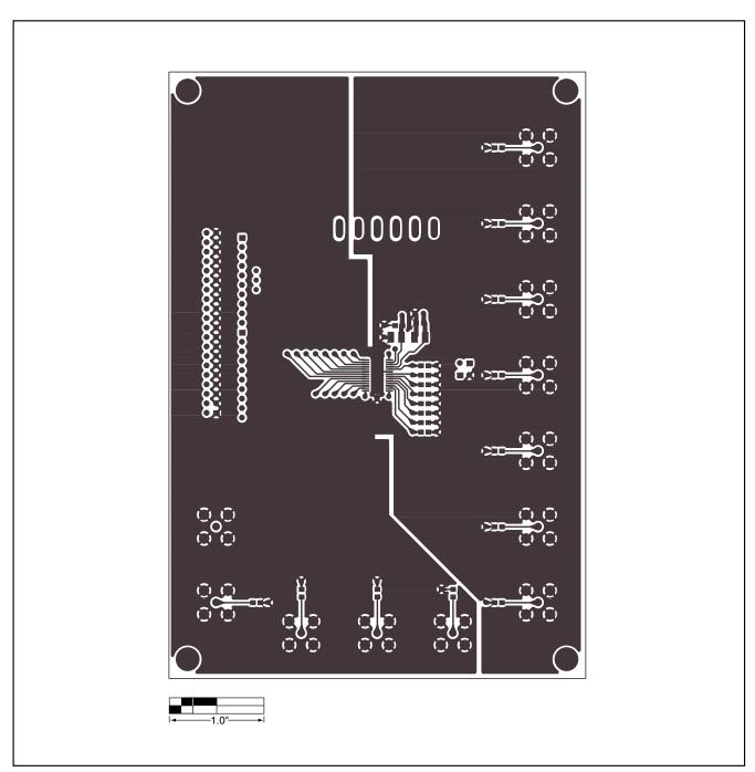
Figure 3. MAX1294 EV Kit PC Board Layout—Component Side
