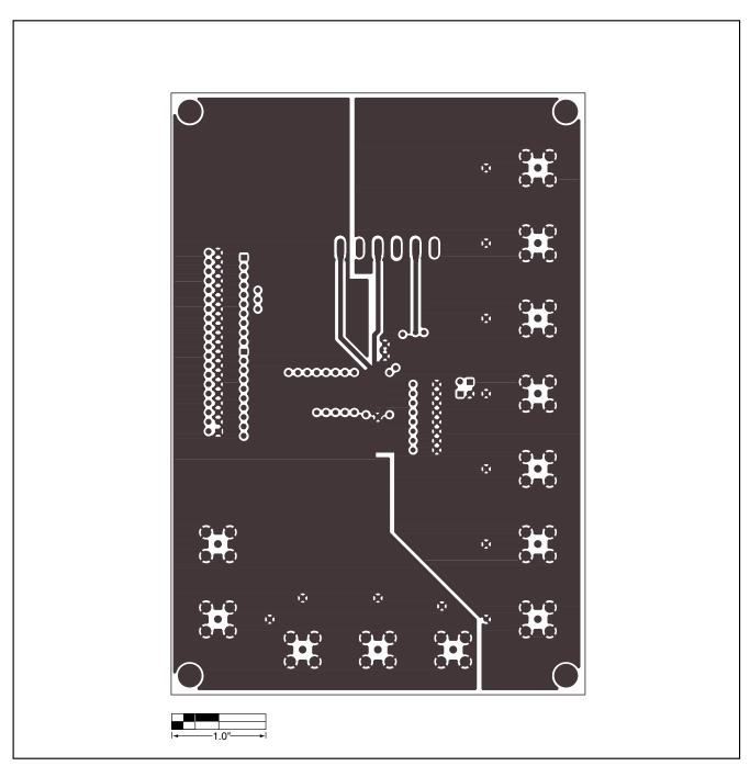
Figure 5. MAX1294 EV Kit PC Board Layout—Interior Layer 2
