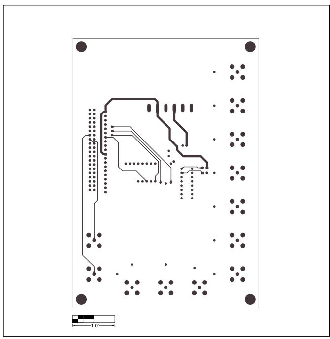
Figure 4. MAX1294 EV Kit PC Board Layout—Interior Layer 1
