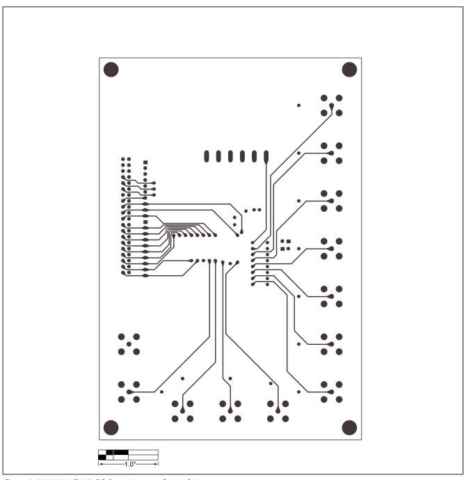
Figure 6. MAX1294 EV Kit PC Board Layout—Solder Side
