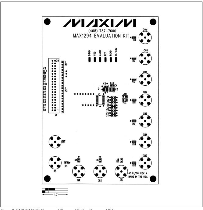
Figure 2. MAX1294 EV Kit Component Placement Guide—Component Side
