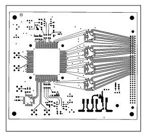
Figure 5. MAX101A EV Kit Main Board Layout—Layer 1
