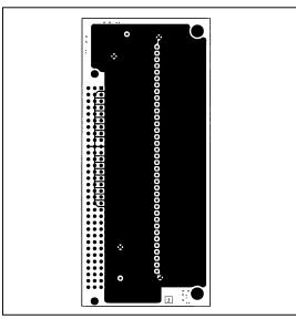
Figure 16. MAX101A EV Kit Termination Board Layout—Layer 3
