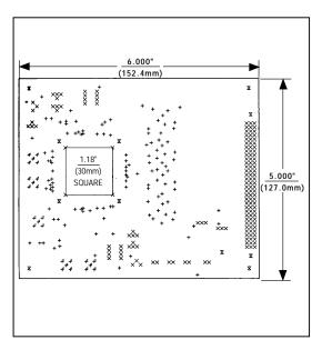
Figure 11. MAX101A EV Kit Main Board Mechanical Guide
