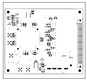
Figure 4. MAX101A EV Kit Main Board Component Placement Guide—Solder Side
