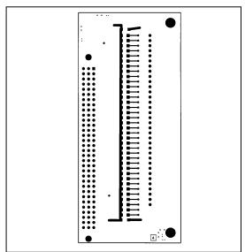
Figure 17. MAX101A EV Kit Termination Board Layout—Layer 4
