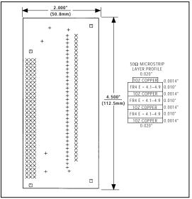
Figure 18. MAX101A EV Kit Termination Board Mechanical Guide
