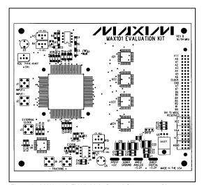
Figure 3. MAX101A EV Kit Main Board Component Placement Guide—Component Side
