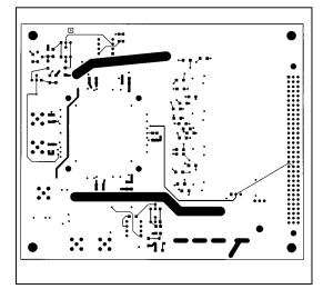
Figure 10. MAX101A EV Kit Main Board Layout—Layer 6
