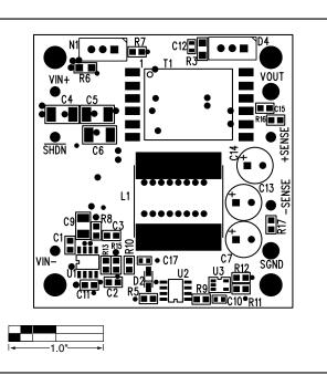
Figure 5. MAX5015 EV Kit Component Placement Guide— Component Side
