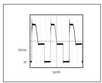
Figure 3. MOSFET N1, Drain-Source Voltage Waveform, VIN+ = 48V
