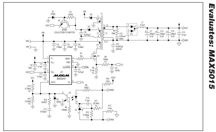
Figure 4. MAX5015 EV Kit Schematic
