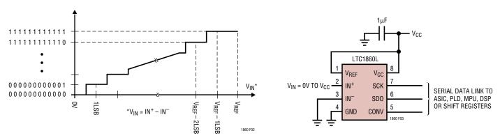
Figure 2. LTC1860L Transfer Curve
