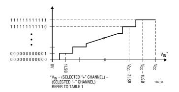
Figure 5. LTC1861L Transfer Curve
