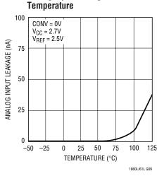
Analog Input Leakage vs
