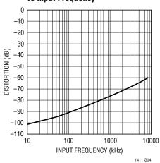
S/(N + D) vs Input Frequency and Amplitude
