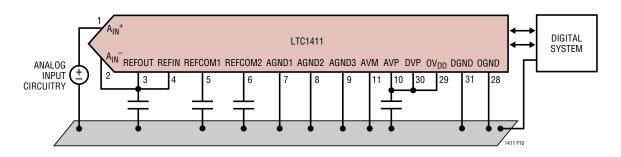
Figure 10. Power Supply Grounding Practice
