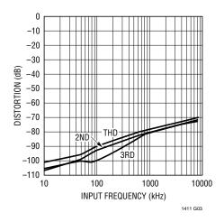
Figure 4. Distortion vs Input Frequency
