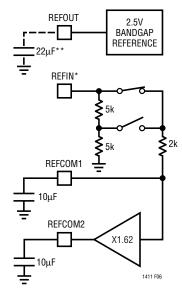
\*THIS PIN CAN BE TIED TO REFOUT OR AN EXTERNAL SOURCE \*\*A  $22\mu F$  CAPACITOR IS NEEDED IF REFOUT IS USED TO DRIVE  $A_{1N}^-$
