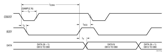
Figure 11a. CONVST Starts a Conversion with a Short Active Low Pulse
