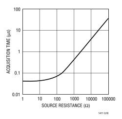
Figure 5. Acquisition Time vs Source Resistance
