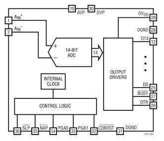
Figure 1. Simplified Block Diagram
