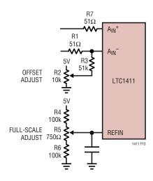
Figure 13. Offset and Full-Scale Adjustment
