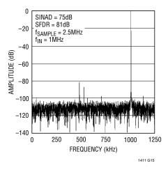
Figure 2b. LTC1411 4096 Point FFT, Input Frequency = 1MHz
