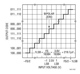
Figure 12. LTC1411 Bipolar Transfer Characteristics (2's Complement)
