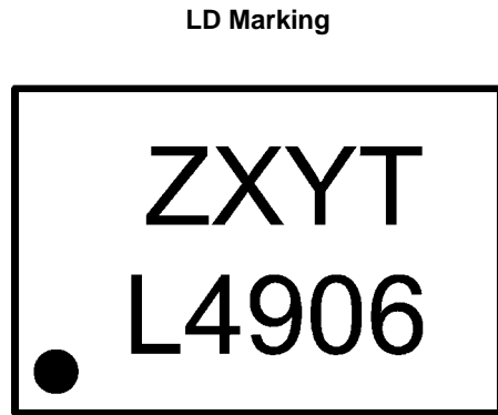
Z - Plant Code XY - Date Code T - Die Traceability
