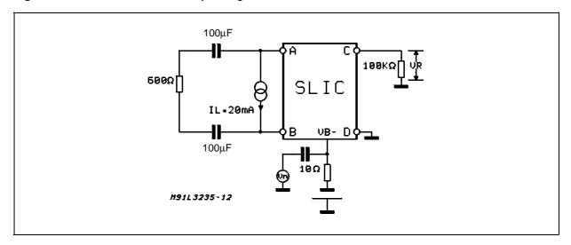
Figure A6: Longitudinal to Transversal Conversion
