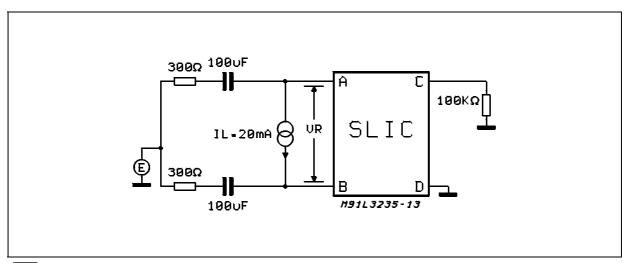
Figure A7: Transversal to Longitudinal Conversion
