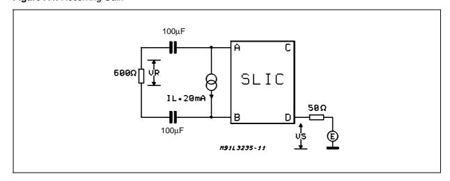
Figure A5: SVRR Relative to Battery Voltage VB
