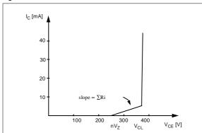
FIGURE 3: V<sub>cl</sub> with load L≅4mH
