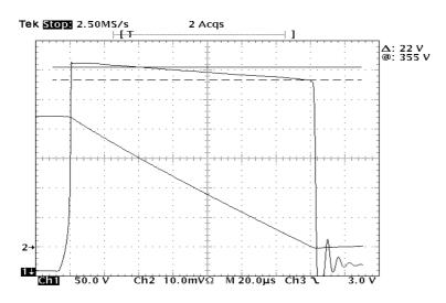
FIGURE 4: Output Current Waveform after Thermal Protection Activation.
